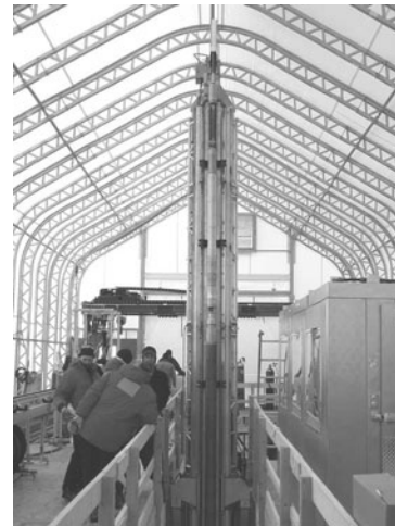
Fig. 8. Drill tower with sonde.
