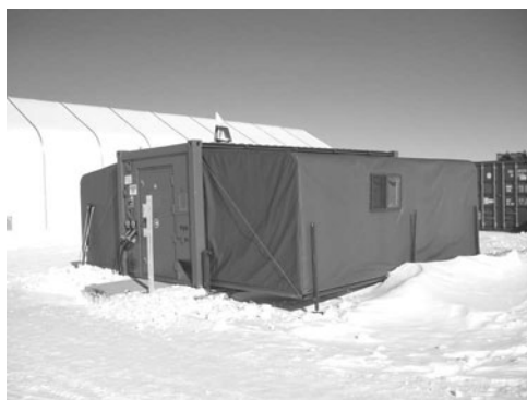
Fig. 13. The MECC container that houses the shop; the sections to the right front and left rear collapse into the center section for shipping.
