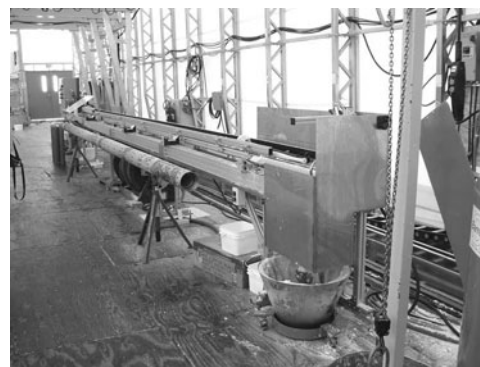
Fig. 12. Screen-cleaning station; a screen section is laid out to the left of the barrels.
