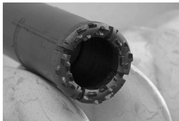
Fig. 5. Temperature-stabilized diamond rock-coring bit.
