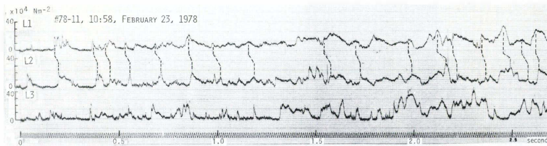
Fig. 7. Internal wave fronts of avalanche No. 78-11. Load cells L2 and L3 were 45 cm and 5 m in down-stream of L1, respectively (Shiai-dani).
