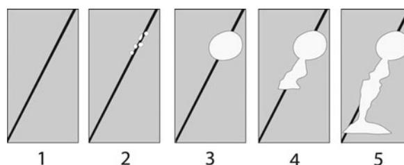
**Fig. 10.** Conceptual model of conduit evolution. 1: Debris-filled crevasse trace (aligned perpendicular to the page); 2: water flow creates network of proto-conduits; 3: elliptical phreatic tube; 4: vadose incision of conduit floor towards local base level; 5: incision becomes independent of parent structure, and passage floor stabilizes at base level.
