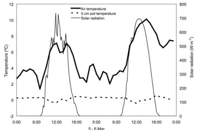
**Fig. 7.** Meteorological conditions on the northeast-facing slope of the Treeline site during the period shown in Figure 6. Soil temperature measurements were made with type T thermocouples referenced to a thermistor with an accuracy of  $0.5^{\circ}\text{C}$ .
