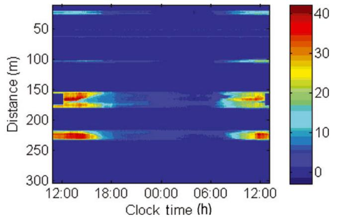
**Fig. 4.** Time-lapse image of the basal snow temperatures along the Mammoth cable. The two warmest sections are the areas where the fiber crossed bare ground. Short sections of the fiber were also exposed at  $\sim 20$  and  $\sim 100$  m and show as warm areas during midday. The circled portions of the graph indicate that portion of the fiber placed in the ice/slush bath for calibration.
