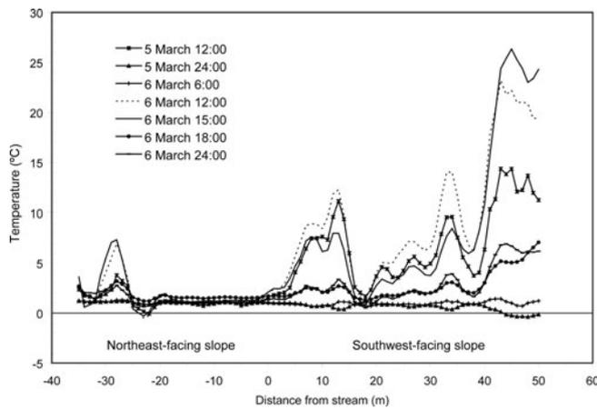
**Fig. 6.** Temperature distribution at the snow/soil interface across the Treeline site during a 36 hour period of active melting. The 0 m position is in the valley bottom stream. Negative numbers on the x axis advance up the north-facing slope, and positive numbers advance up the south-facing slope. Positions  $-30$  m and  $+45$  m are on relatively flat ridges.
