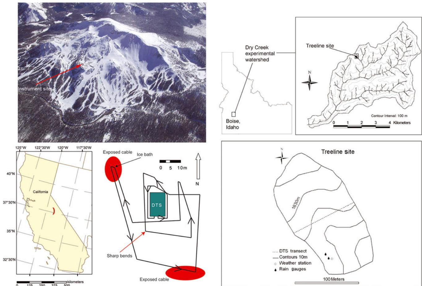
**Fig. 2.** Plan views of the two instrument sites, showing fiber deployment pattern. (a) Mammoth Mountain site, where the fiber is highlighted in red for those portions that traversed bare ground; and (b) DCEW.
