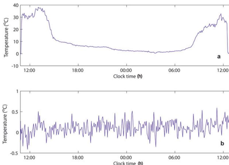
**Fig. 5.** Temporal changes in temperature at Mammoth Mountain: (a) cable located on bare ground; and (b) cable located at the snow/soil interface. Note the different temperature scales in the two graphs.
