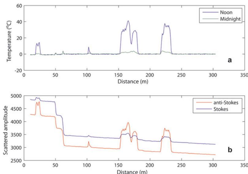
**Fig. 1.** Typical temperature (a) and Raman-scattering signals (b) from a fiber-optic cable during snowmelt. (a) demonstrates the ability of the system to detect large temperature changes over short distances; (b) shows the impact of temperature on the ratio of the Stokes and anti-Stokes scattered signal. The step changes in amplitude at 50 and 60 m in (b) represent attenuations caused by sharp bends or kinks in the cable.
