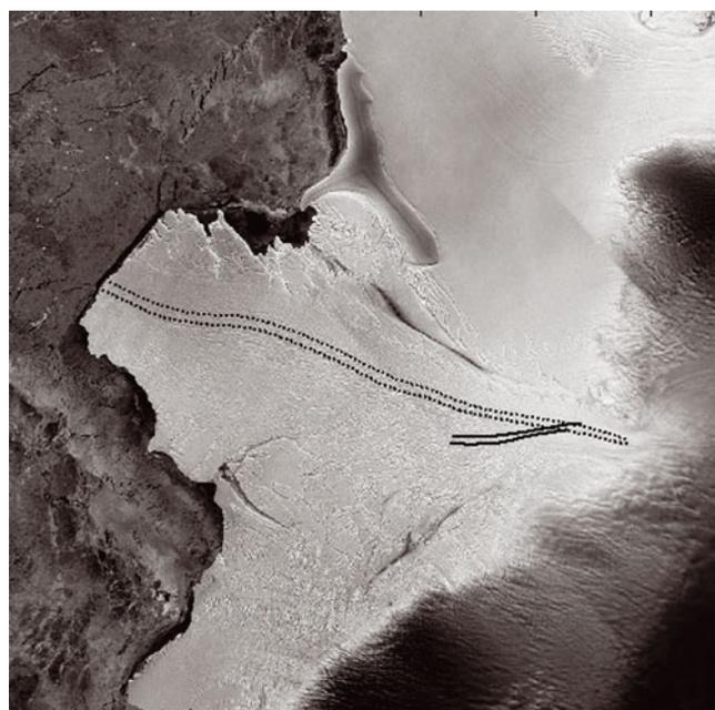
**Fig. 5.** Reconstructed configuration of two relict flow stripes at the approximate time of perturbation (solid lines), ~137 years earlier, and position of the stripes on a 1997 image (dotted line). The extrapolation makes use of the derived velocity field (Fig. 2) to estimate the configuration in the past. The reconstruction indicates that flow-stripe bending was more extreme in the past and has since stretched out as a result of velocity gradients along the ice tongue.
