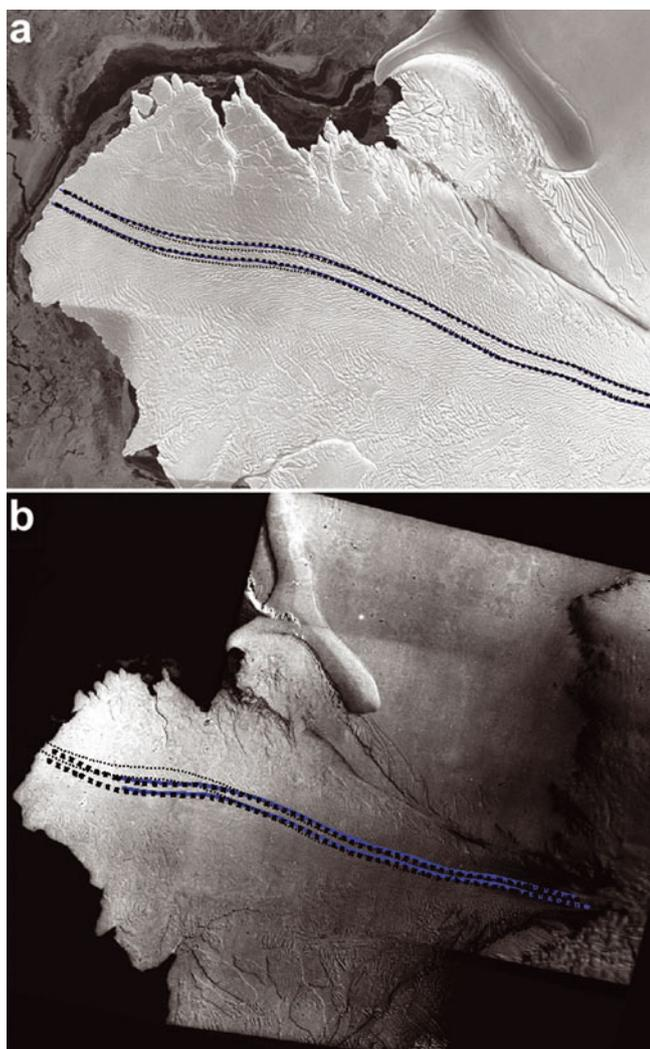
**Fig. 4.** Comparison between extrapolated relict flow stripes (thick dotted line) and actual position of the same flowlines (blue) on (a) a 2000 RADARSAT image and (b) a 1986 Landsat image. The thin dotted line gives the 1997 position of the same flow stripes. The good agreement indicates that flow has been relatively constant since 1986.
