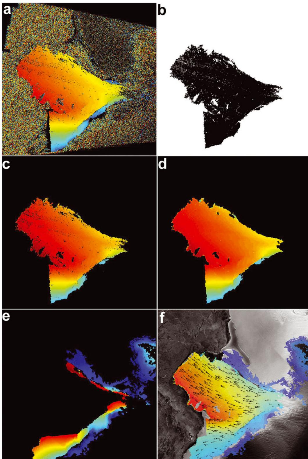
**Fig. 1.** Ice-flow velocity on the BIS and SWIT. (a) Unfiltered IMCORR output of fast flow; (b) mask created by a region-growing technique; (c) output after the mask is applied; (d) output after leftover outliers are filtered out and small gaps are filled in using an inverse distance-weighted standard deviation filter; (e) filtered output of slow flow; and (f) merged fast and slow velocity field projected on a RADARSAT-1 image with some vectors displayed.
