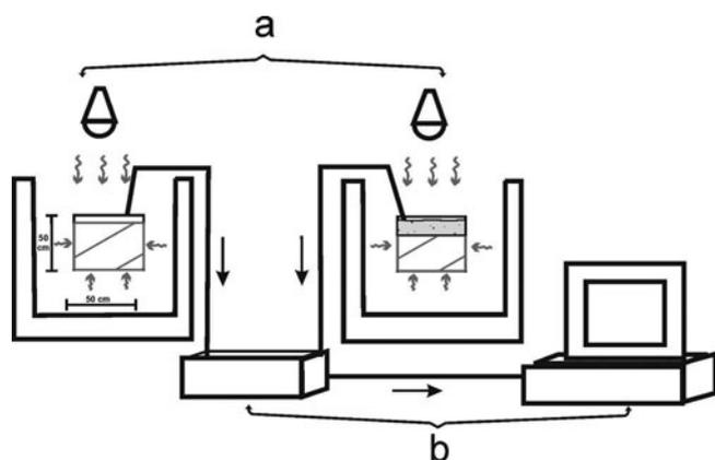
**Fig. 2.** The experimental arrangement for tests with diurnal cycles: (a) melting blocks of bare and debris-covered ice exposed to identical radiation during the 12 hour ablation period (attained by two electric bulbs with short- and longwave radiation, shown by grey lines) and cooling by freezer during the 12 hour night (shown by black lines); (b) Campbell Scientific 21X data logger and PC, which recorded temperature and heat-flux profiles.
