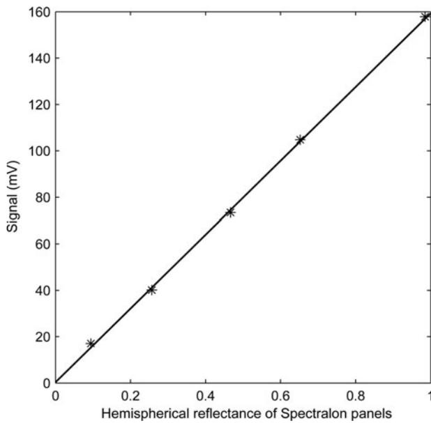
**Fig. 3.** Measured signal of the +20° photodiode for five different calibration panels. The reflectance of the calibration panels is the hemispherical reflectance at 1310 nm. The trend is the least-square linear regression.
