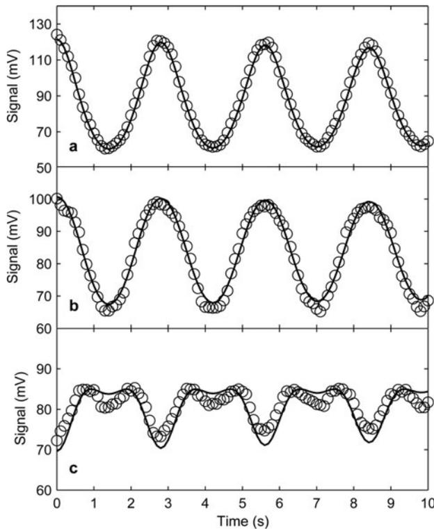
**Fig. 4.** Effect of the distance between the point of convergence of the photodiodes and the reflecting surface (Spectralon 50%) on the measured signal for the 20° (a), 40° (b) and 60° (c) photodiodes (circles). The horizontal displacement was varied from -12 mm to +12 mm relative to the ideal distance. Signals calculated (solid curves) with Equations (8–11) are compared to the experimental data.
