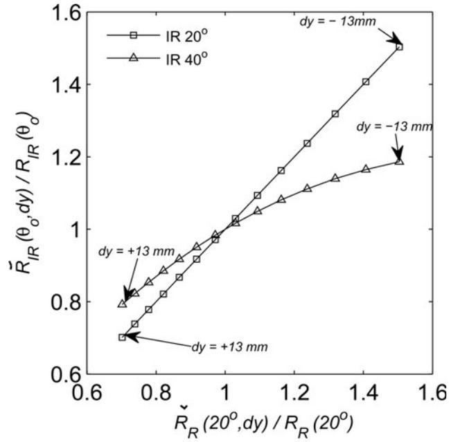
**Fig. 6.** Variations of  $\tilde{R}_{IR}(\theta_0, dy)/R_{IR}(\theta_0)$  versus  $\tilde{R}_R(20^\circ, dy)/R_R(20^\circ)$  at two different viewing zenith angles,  $\theta_0$  ( $20^\circ$  and  $40^\circ$ ), calculated using the geometrical model for variations of  $dy$  in the range  $\pm 13$  mm.
