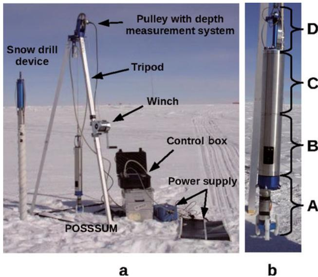
**Fig. 1.** (a) Experimental set-up in the field with POSSUM, the snow drill device, the tripod with a manual winch and a depth system measurement, the data acquisition system and the power supply. (b) Picture of POSSUM which is composed of a bore with a guiding system (A), an optical measurement part with laser diodes and photodiodes (B), an electronic part for laser drivers and photodiode amplifiers (C) and anti-torque system (D).
