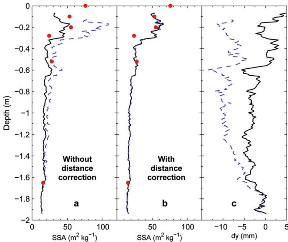
**Fig. 12.** Profiles of SSA obtained with POSSSUM on Glacier de la Girose on 17 April 2009 without (a) and with (b) distance correction during the descent (solid curves) and the ascent (blue dashed curves). To quantify the distance correction during descent and ascent, the distance  $dy$  calculated with Equations (12–16) is plotted (c). Some SSA measurements using methane adsorption on sampled snow (red circles) are also shown for direct comparison.
