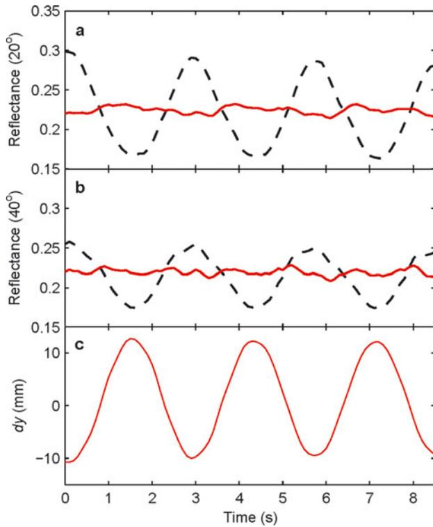
**Fig. 7.** Effect of the distance correction on the reflectance at two different viewing zenith angles: (a)  $20^\circ$  and (b)  $40^\circ$ . Dashed curves are snow reflectances during the pendulum experiment, and red solid curves are the distance-corrected signals. (c) Amplitude of the oscillations of POSSSUM  $dy$  calculated with the reflectance measured at 635 nm and Equation (12).
