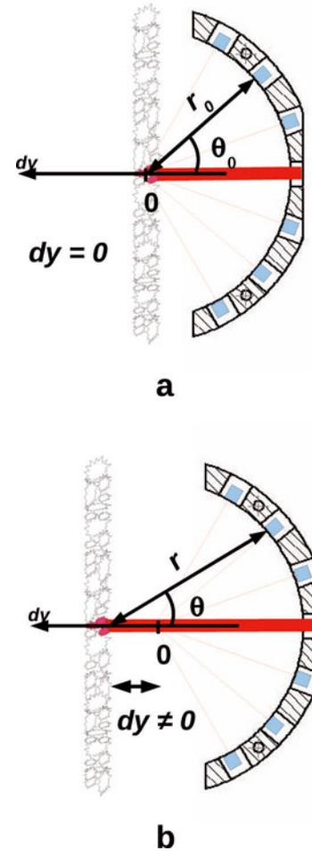
**Fig. 5.** Two geometrical configurations of POSSUM's optical head in the hole and parameters used in the calculation of the power received by the photodiode as a function of the distance  $dy$ . (a)  $dy=0$  ideal position (i.e. no correction needed) and (b)  $dy \neq 0$  position implying a distance correction.
