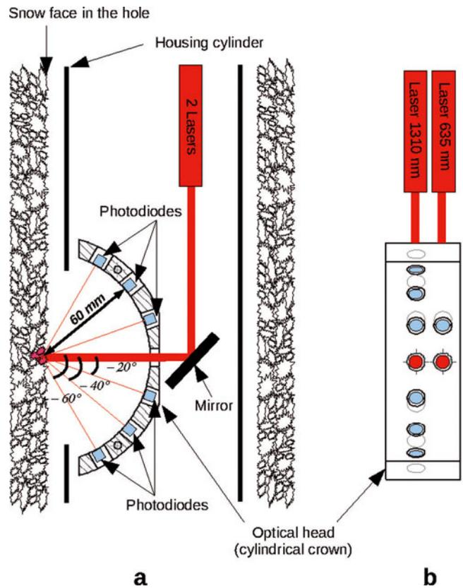
**Fig. 2.** Schematic view of the optical system of POSSUM showing the relative positions of illumination source (laser) and reflectance measurements (photodiodes): (a) side view; (b) front view, in the axis of the illuminating beam.
