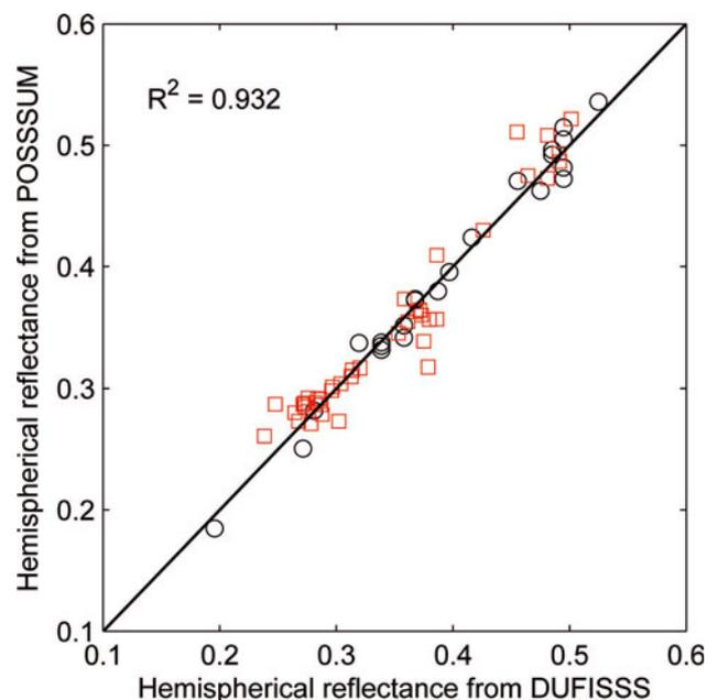
**Fig. 10.** Comparison of hemispherical reflectances obtained with POSSUM and DUFISSS. Squares are field measurements, and circles are laboratory measurements.  $R^2$  is computed with the residual sum of squares errors between the real data points and the  $y=x$  model.
