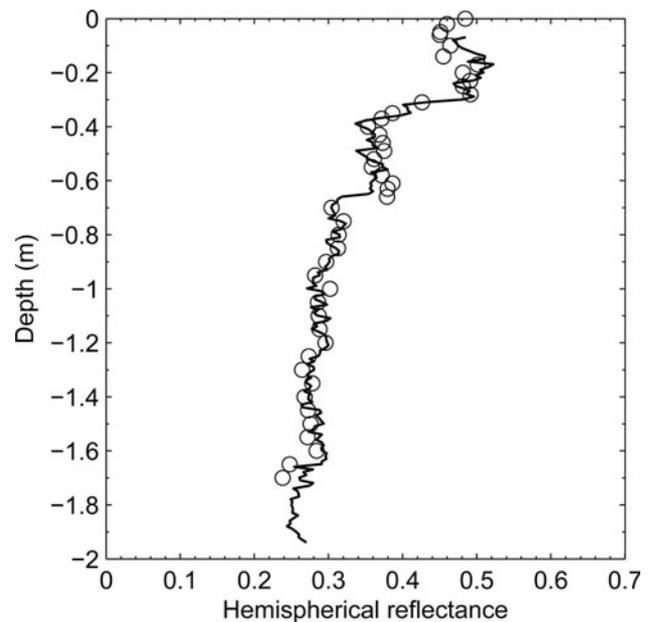
**Fig. 9.** Profiles of hemispherical reflectance measured with POSSUM (solid line) and discontinuous measurements with DUFISSS (circles) obtained on Glacier de la Girose on 17 April 2009.
