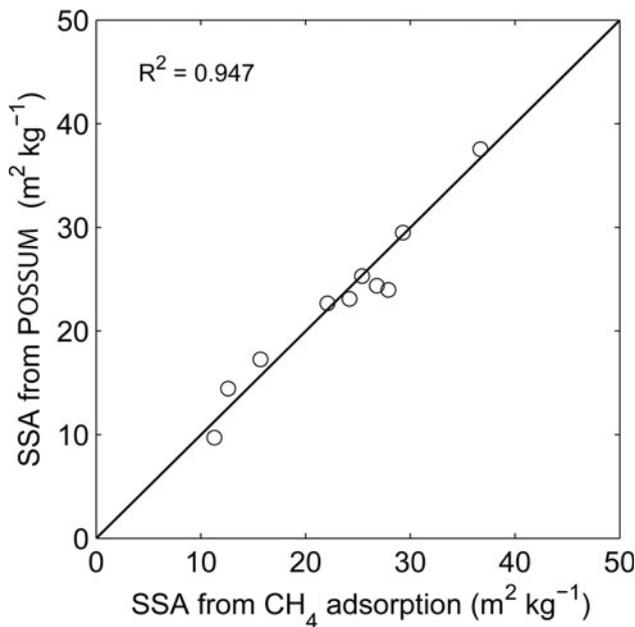
**Fig. 11.** SSA calculated with the processing algorithm from the reflectance measured with POSSSUM versus SSA measured using CH<sub>4</sub> adsorption at 77 K.  $R^2$  is computed with the residual sum of squares errors between the real data points and the  $y=x$  model.
