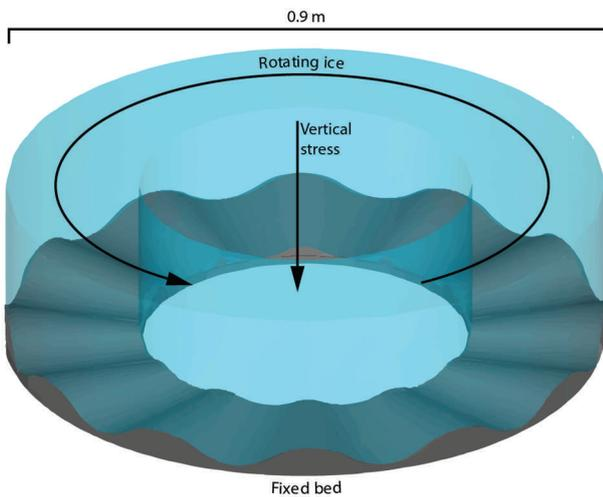
**Fig. 1.** Schematic of the ice ring and sinusoidal bed. An annular plate with teeth grips the upper surface of the ring and drags it across the bed. The ring also slides along smooth walls that confine it along its sides. See Iverson and Petersen (2011) for more details.
