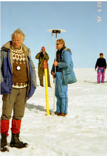
First attempt to survey location and elevation of a mass balance survey site with kinematic GPS, with ~10 cm accuracy in 1992. Helgi Björnsson (left), Magnús Tumi Guðmundsson holding antenna; both long term presidents of the society. Páll Einarsson, seismologist, taking a photograph of the setup of his GPS instrument. Photo: Finnur Pálsson.
