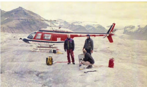
Drilling a 15 m hole with a steam drill to install a wire to measure summer ablation on the snout of Skeiðarárjökull in 1997. Photo: Finnur Pálsson.
