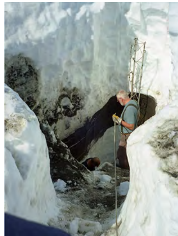
Digging out the instrument mast in Grímsvötn in June 1999 (~8 m). The instruments measured the water level of the lake and relayed data to Reykjavík. The instruments broke down during the Grímsvötn eruption in December 1998. The ~1 m thick tephra layer was tough as concrete. Photo: Finnur Pálsson.
