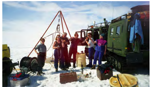
Hot water drill used to drill through the ~300 m thick floating ice shelf of Grímsvötn lake to sample the lake water in June 1998. Happy drillers toasting after hitting through. Photo: Finnur Pálsson.
