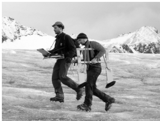
Figure 1. Radar sounding of the subglacial drainage system of the frontal part of Werenskiöld glacier by Darek Puczko and Mariusz Grabiec in the autumn of 2007 (Photo J. Jania)
