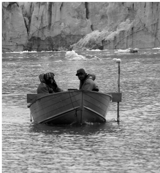
Figure 3. Acoustic echo-sounding of the depth of the bay at the foot of Recherchebreen (a tidewater glacier in southwest Spitsbergen) in summer 2008 (Photo P. Zagórski)
