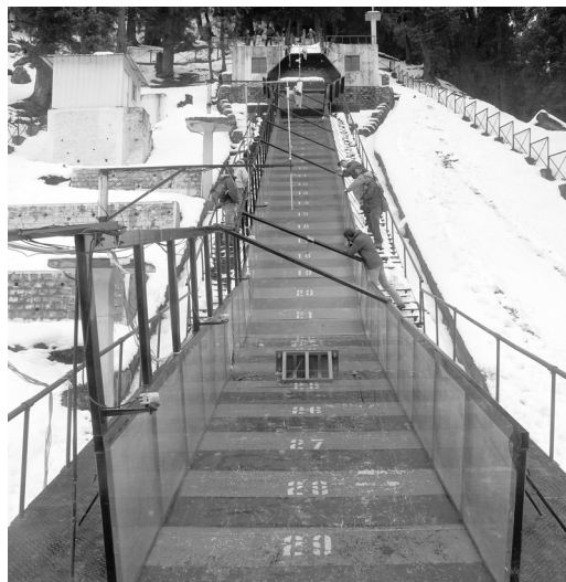
Fig. 6. Here comes the snow, here comes the snow... An instrumented avalanche on the avalanche chute of the Dundhe Snow Research Station of SASE.
